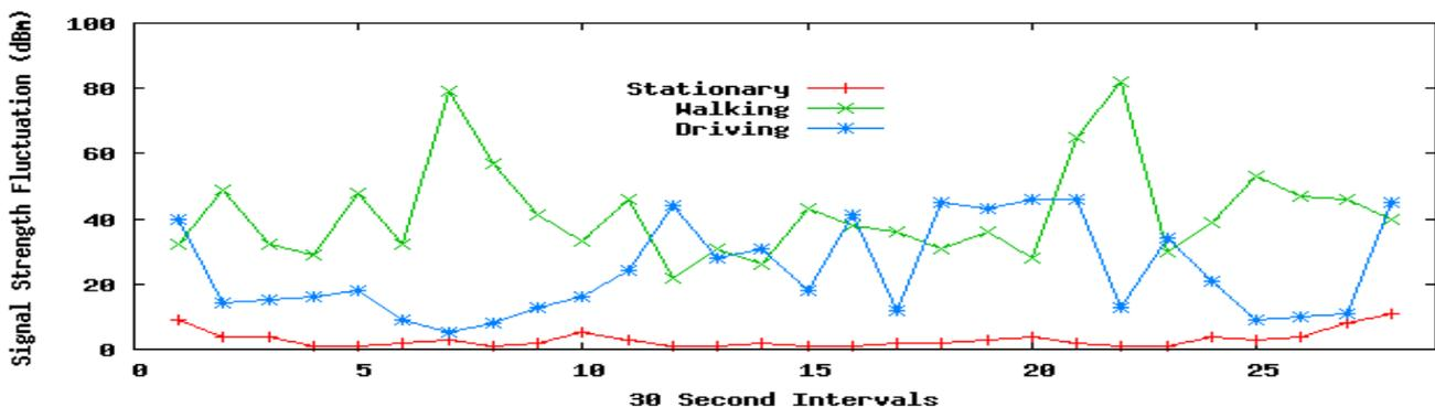
Figure 2: Distinguishable patterns of GSM signal strength fluctuation over successive 30 second samples are used in identifying the activity levels *Stationary*, *Walking* and *Driving*.
